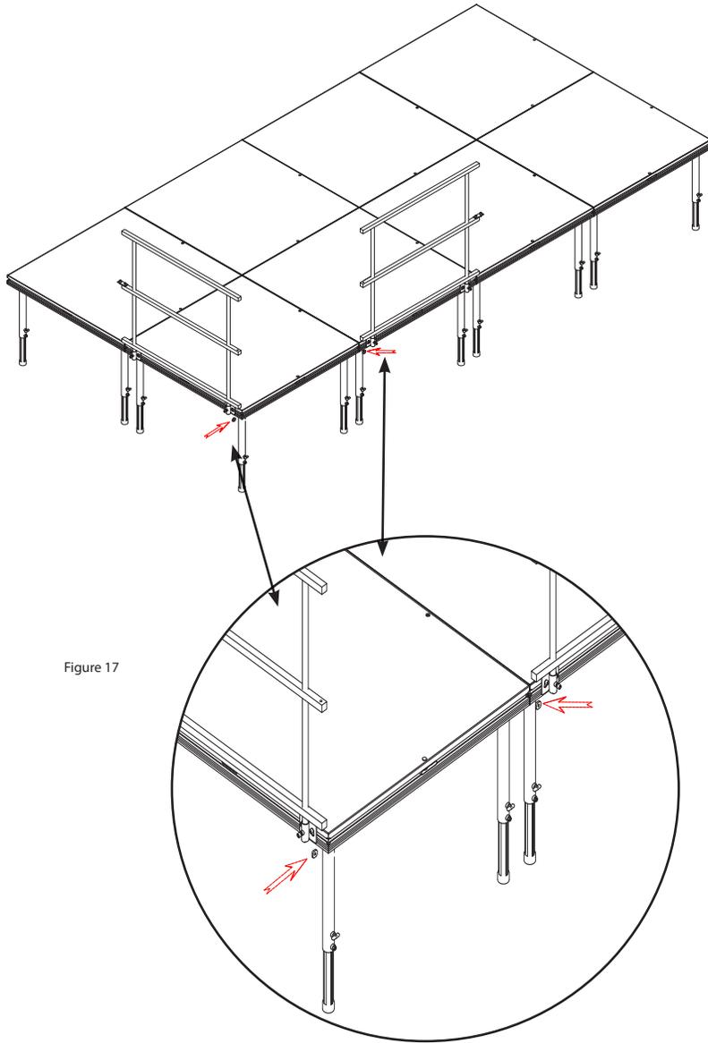
Slide assembly inserts into QuickLock platform as shown in figure 17
