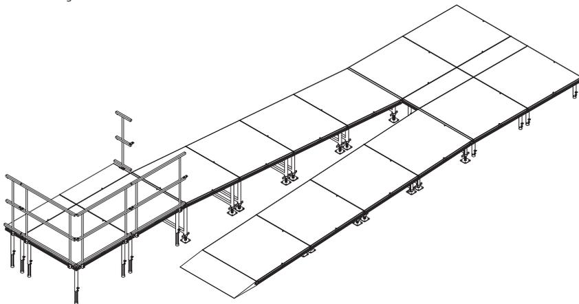
Attach RAGRD4, QLGRS4 and RASGRD guardrails together by sliding extension tubes into the openings on both guardrails as shown in the drawing and securing them with hardware as shown in figures 35 thru figure 38
