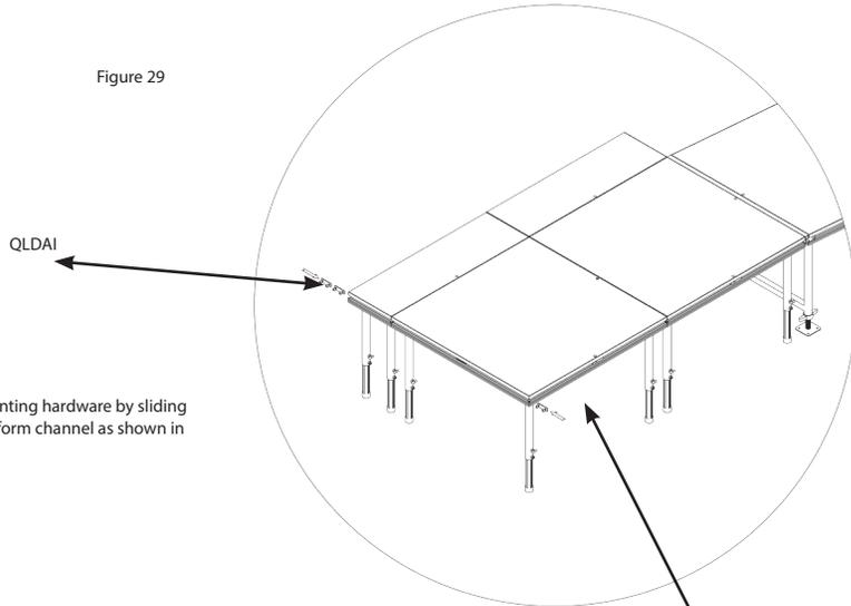
Insert guardrail mounting hardware by sliding it into the stage platform channel as shown in figure 29
