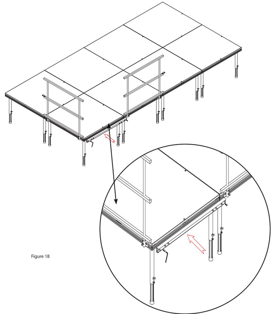
Attach RRUCP/RRUCPAL connecting panel to stage platform with included hardware and hex key as shown in figure 18
