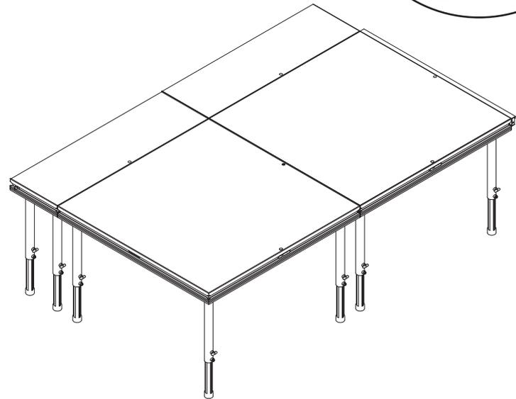
Next attach the platform with the installed stage connecting panel ( RUCP or RUCPAL ) to the top ramp platform with provided hardware as shown in figure 12
