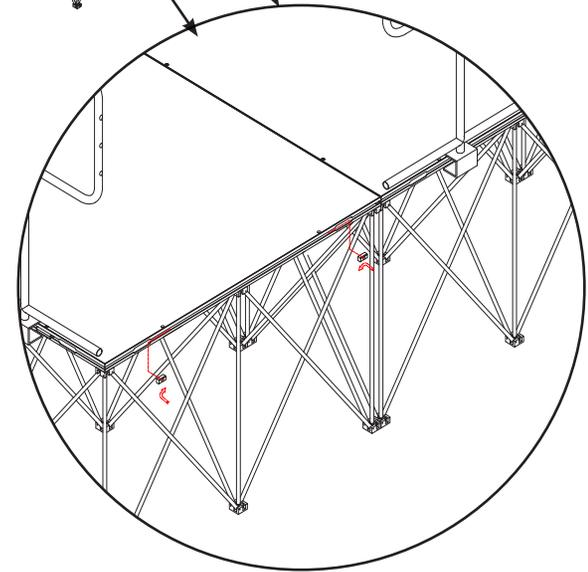
Slide assembly inserts into Intellistage platform as shown in figure 14
