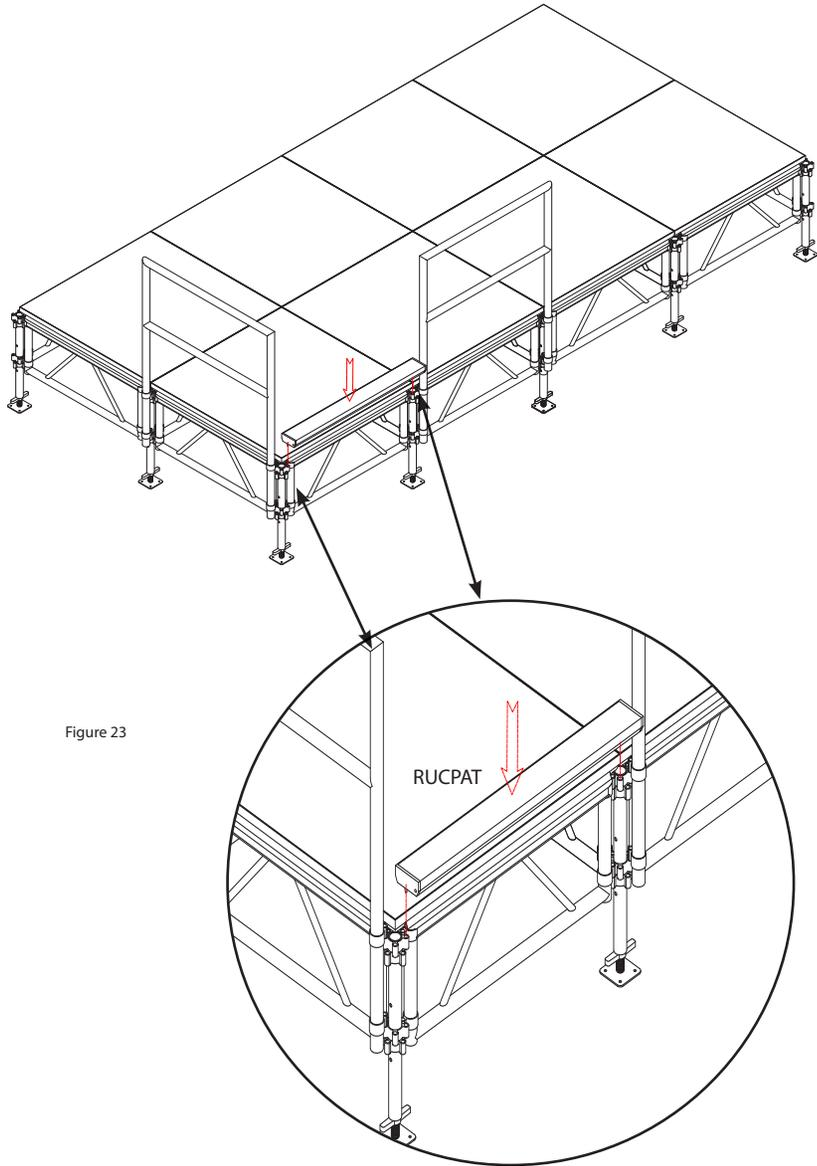
Attach RUCPAT connecting panel to stage platform as shown in figure 23
