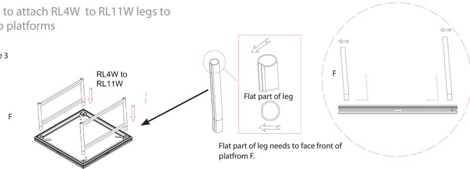
Start with platform upside down and with Quick Lock mechanisms open as shown in step 1. Place legs into the locking mechanisms of platform as shown in step 2. The flat part of the leg needs to face the front of the platform F as shown in figure 3. Close the Locking mechanism to secure legs into the bottom of the platform as shown in step 2. Set platform right side up and place onto height adjustable feet as shown in steps 3 and 4.
