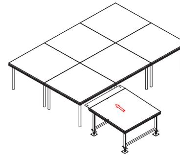
Place top ramp platform with installed stage connecting panel next to surface you would like to attach the ramp too
