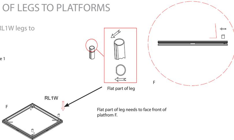
Start with platform upside down and with Quick Lock mechanisms open as shown in step 1. Place legs into the locking mechanisms of platform as shown in step 2. The flat part of the leg needs to face the front of the platform F as shown in Figure 1. Close the Locking mechanism to secure legs into the bottom of the platform as shown in step 2. Set platform right side up and place onto height adjustable feet as shown in steps 3 and 4.
