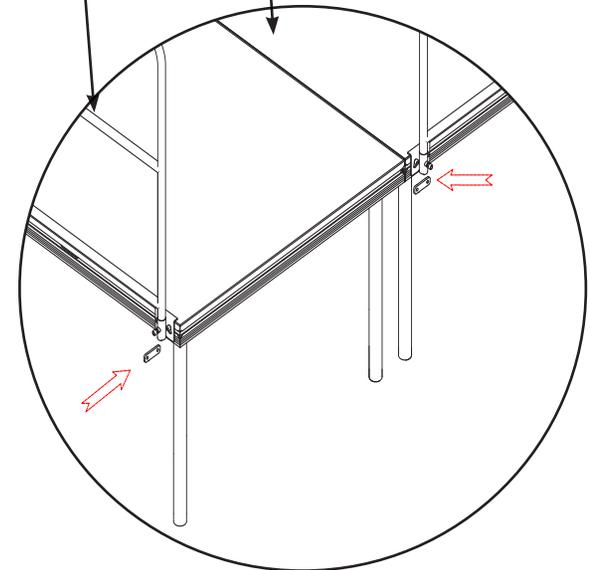
Slide assembly inserts into ProFlex platform as shown in figure 20
