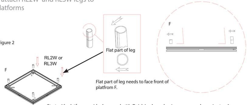
Start with platform upside down and with Quick Lock mechanisms open as shown in step 1. Place legs into the locking mechanisms of platform as shown in step 2. The flat part of the leg needs to face the front of the platform F as shown in figure 2. Close the Locking mechanism to secure legs into the bottom of the platform as shown in step 2. Set platform right side up and place onto height adjustable feet as shown in steps 3 and 4.
