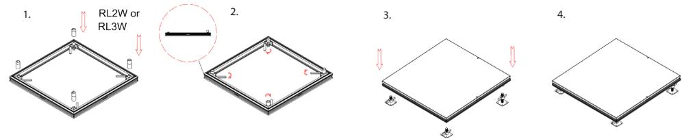
How to attach RL4W to RL11W legs to ramp platforms
