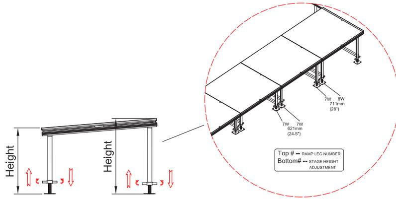
Adjust bottom of ramp legs by turning
