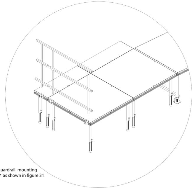
Insert guardrails into guardrail mounting hardware OLGRCCLAMP as shown in figure 31
