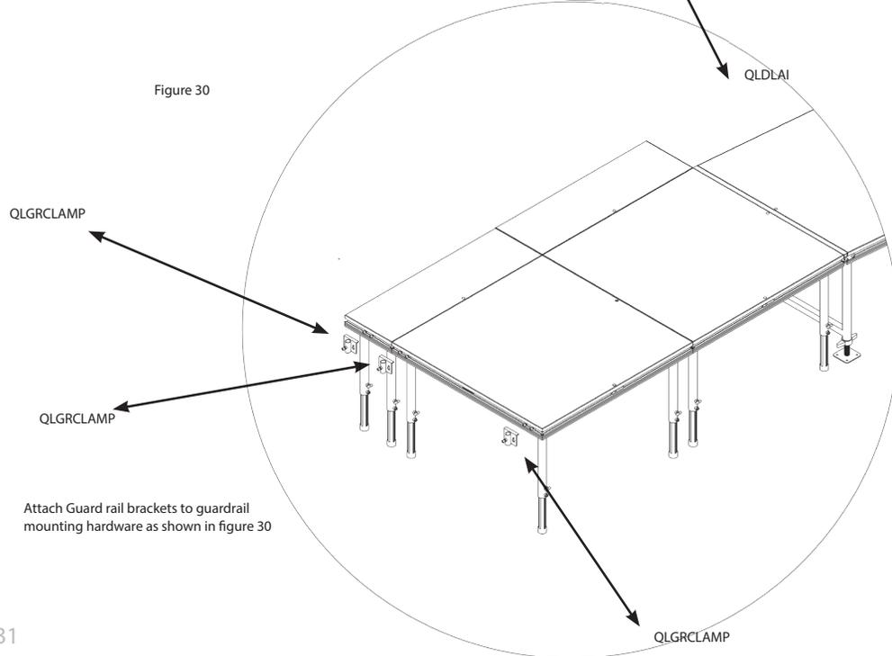
Attach Guard rail brackets to guardrail mounting hardware as shown in figure 30
