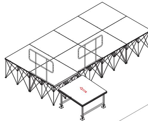
Place top ramp platform to next to installed stage connecting panel
