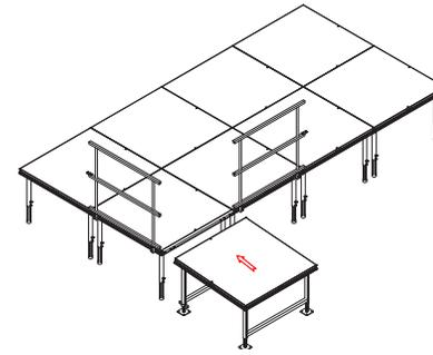
Place top ramp platform next to installed stage connecting panel
