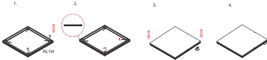
How to attach RL2W and RL3W legs to ramp platforms
