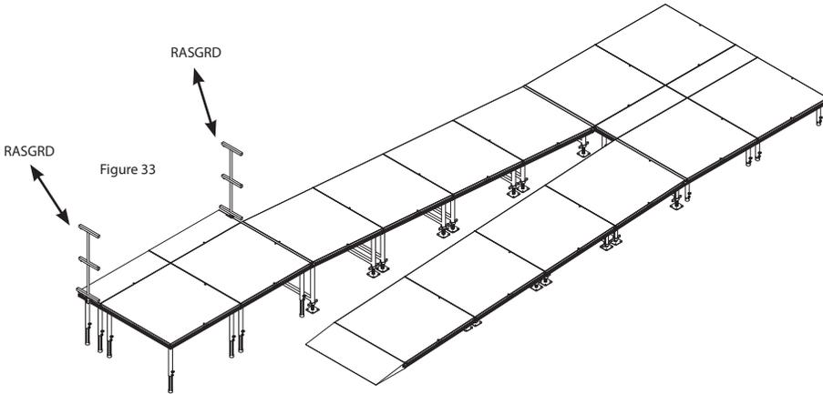
Continue attaching guardrails (QLGRS4) to the platforms as shown in figure 34 with hardware provided following the steps shown in general guardrail assembly in the previous section of this manual.
